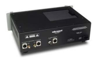
Around back are pairs of single-ended and balanced outputs, S/PDIF BNC and AES/EBU digital outputs, and an IEC power-cord inlet.
