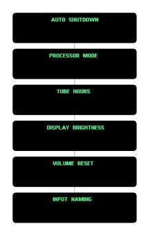
While a menu item is displayed, press 'ENTER', followed by rotating the volume knob on the front panel, or using the volume up/down buttons on the remote to adjust the settings of that particular selection. After making the appropriate change, pressing the 'ENTER' button to choose, then press 'ENTER" again to confirm the new setting; the display will show 'OKAY' for five seconds before reverting back to the normal operation screen.
