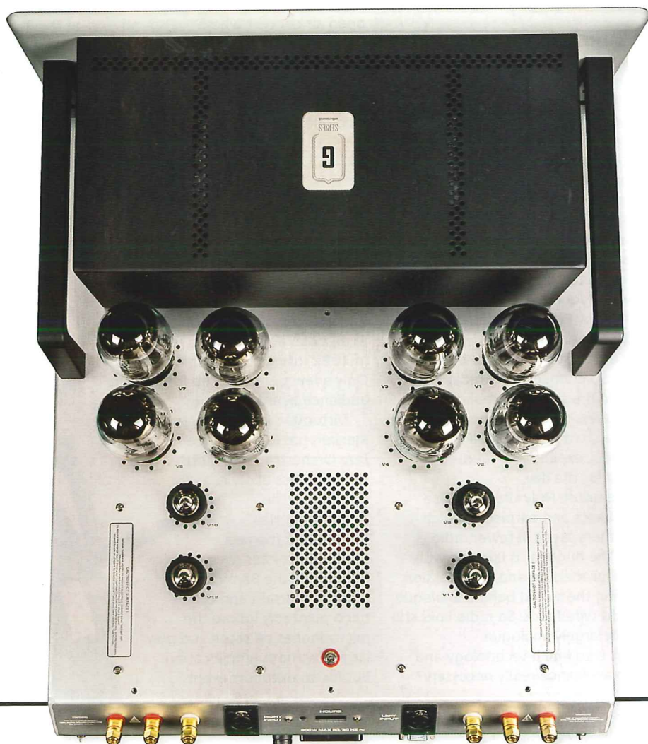
RIGHT: The GS150 features no fewer than two matched pairs of KT150 output tubes per channel driven by pairs of 6H30 double triodes. This is the first ARC amp to use KT150s
